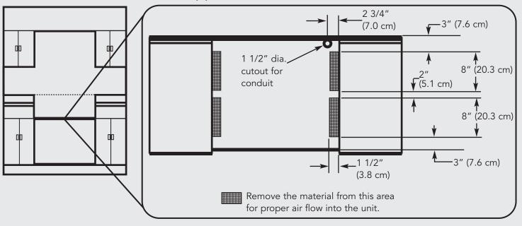
**IMPORTANT:** The electronic components for the induction elements in the rangetop need some air circulation. To ensure long life of electronic components, it is required that a minimum of 8" (20.3 cm) of open space remain between the bottom of the unit and any shelf underneath. The maximum length of the shelf underneath is to be 18" (45.7 cm) There should be no partition or shelf directly underneath the unit.
