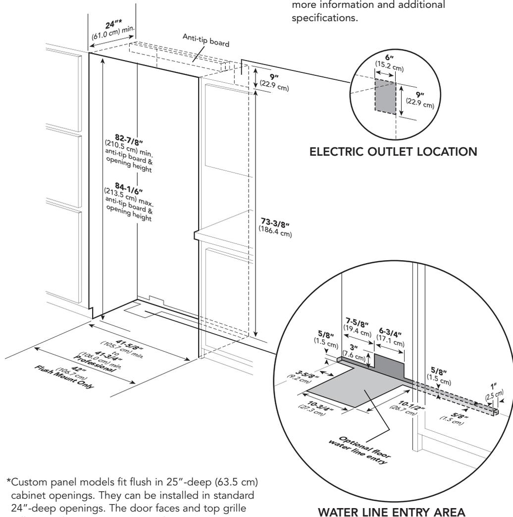
\*Custom panel models fit flush in 25"-deep (63.5 cm) cabinet openings. They can be installed in standard 24"-deep openings. The door faces and top grille will protrude 3/4" (1.9 cm) into the room.
