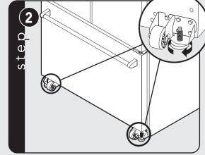
To raise the front of the refrigerator, turn the leveler foot screw clockwise. **Note:** Having someone push against the top of the refrigerator takes some weight off the leveler foot screws.
