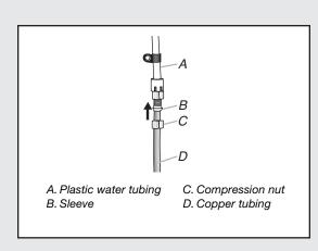
5. Using an adjustable wrench, hold the nut on the plastic water line to keep it from moving. Then, with a second wrench, turn the compression nut on the copper tubing counterclockwise to completely tighten. **DO NOT** overtighten.
