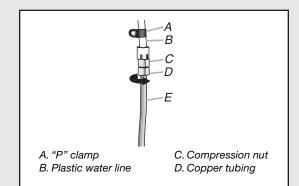
6. Check connection by pulling on copper tubing. Attach copper tubing to refrigerator cabinet with a "P" clamp. Turn on water supply to refrigerator and check for leaks. Correct any leaks.
