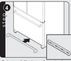
Replace toe grill. Align the toe grille mounting clips with the lower cabinet slots. Push the toe grille firmly until it snaps into place. Check for level.
