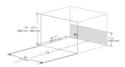
Note: The bottom of the cut-out opening for built-in use must be 36" (91.5 cm) or higher from floor
