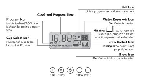
**Note:** If icons continue to blink, the parts are not properly installed and must be removed and properly replaced before brewing begins.
