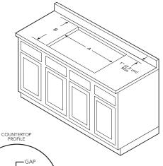
After flush mount installation, if needed, seal the remaining gap with a silicone sealant that is heat-resistant to at least  $320^\circ$ F (160°C). Refer to countertop profile below.
